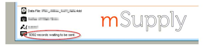
A probable reason for this is that the Sync Satellite server can not connect to the sync Primary server. You can check this by checking the logs (**Special** > **View log...**):
