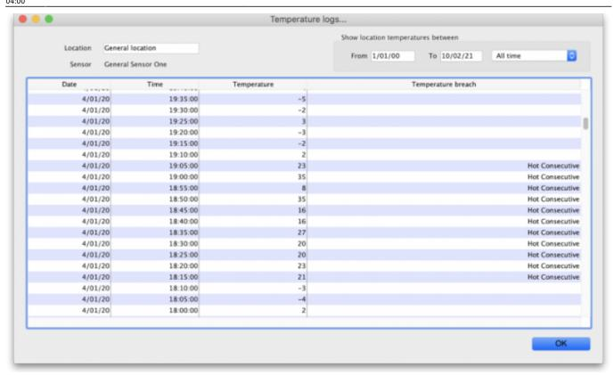
The **Temperature breach** column will contain a description of the breach (e.g. *Hot Consecutive* or *Cold consecutive*) if the log represents a breach, otherwise the column will be empty. So an empty column is good news!
