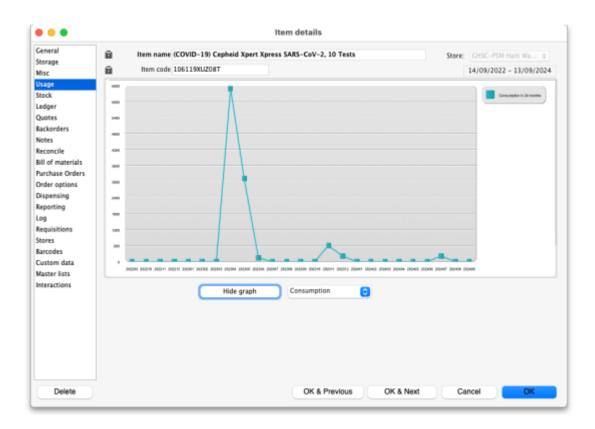
The horizontal (X) axis is the period selected on the **Months** drop down list, the vertical (Y) axis shows the value of the property slected in the drop down list next to the **Show/Hide graph** button
