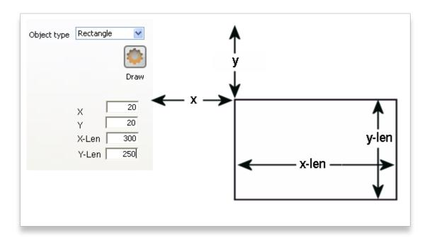
So, as an example, the coordinates are entered as above in the appropriate boxes, then the *Draw* button is clicked to produce the following display under the layout tab:
