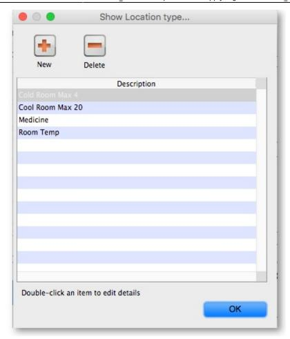
The window that appears allows you to define the criteria for the various types of location in your store - e.g. the permitted temperature range, whether location must be dark, etc.
