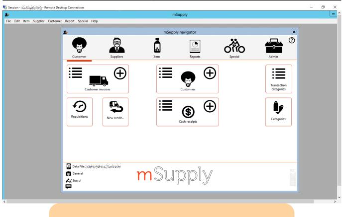
When you're finished, exit mSupply by using the *File*  $\rightarrow$  *Exit mSupply* menu item. If you simply use the *X* button at the top right of the session window, it will close the window but mSupply will continue to run on the server, and use a license which may be needed by someone else.
