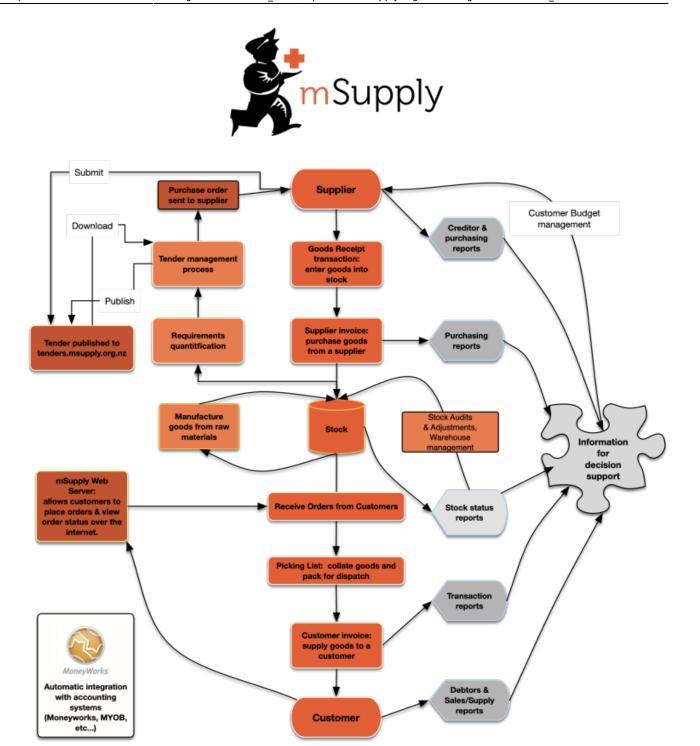
The two most common transaction types in mSupply are the **supplier invoice (si)** and the **customer invoice (ci)**. These transactions record stock purchases from suppliers, and stock supplies to customers respectively. mSupply records stock adjustments through these two transactions. So, given an opening balance of stock, mSupply will show a series of transactions that result in the recorded closing stock.
